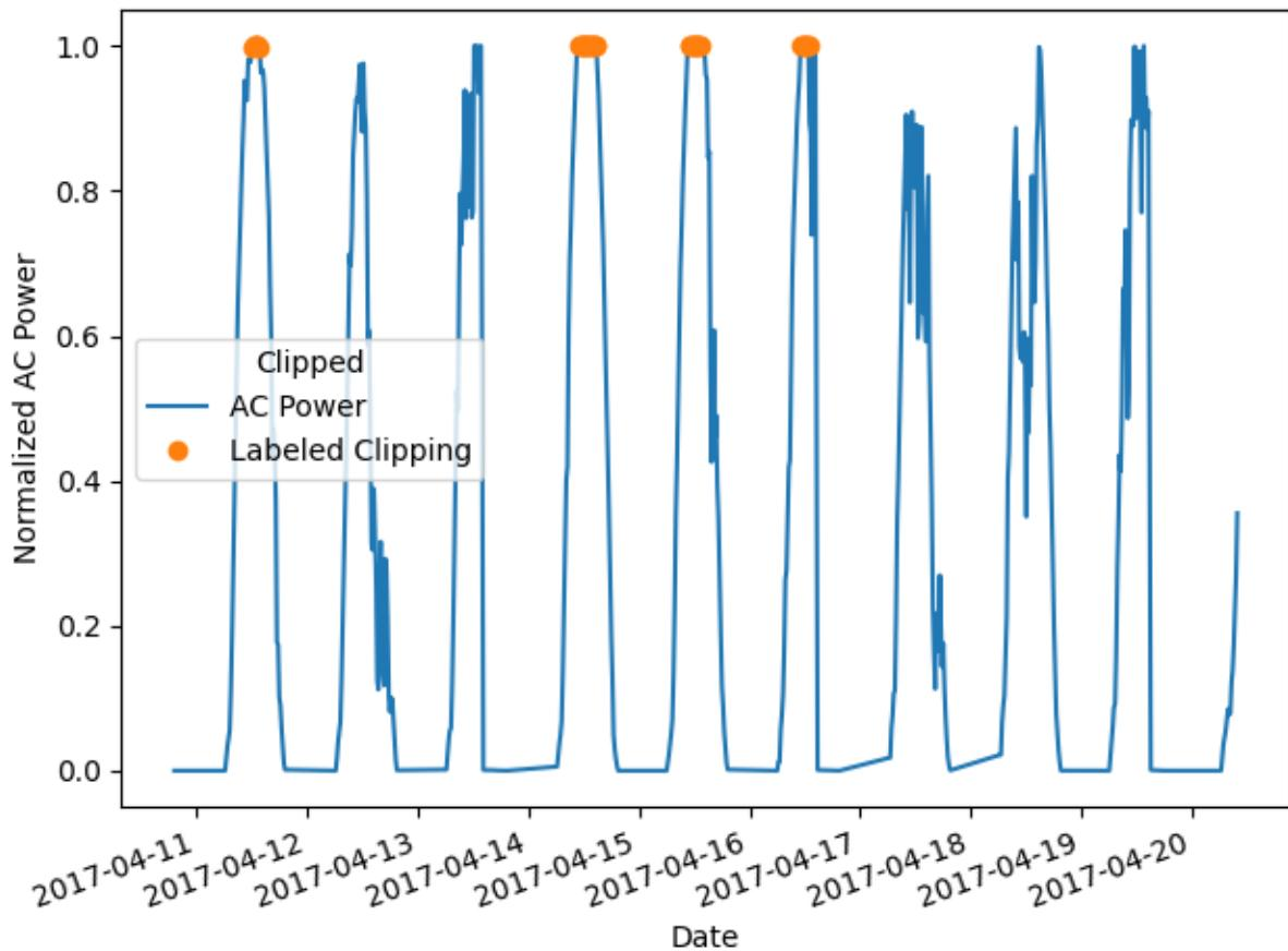
Now, use `pvanalytics.features.clipping.geometric()` to identify clipping periods in the time series. Re-plot the data subset with this mask.
