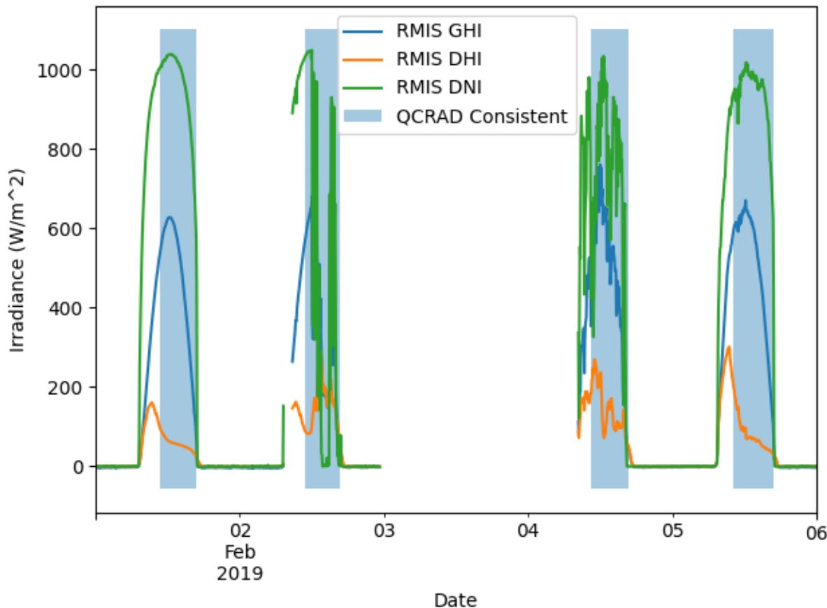
Plot the GHI, DHI, and DNI data streams with the diffuse ratio limit mask overlay. This mask is true when the DHI / GHI ratio passes the limit test.
