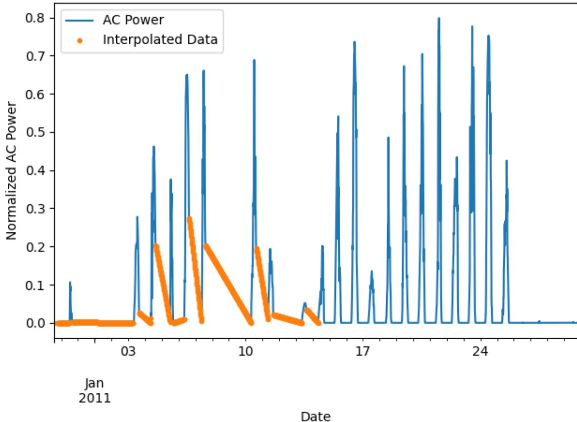
Now, we use `pvanalytics.quality.gaps.interpolation_diff()` to identify linearly interpolated periods in the time series. We re-plot the data with this mask. Please note that nighttime periods generally consist of repeating 0 values; this means that these periods can be linearly interpolated. Consequently, these periods are flagged by `pvanalytics.quality.gaps.interpolation_diff()`.
